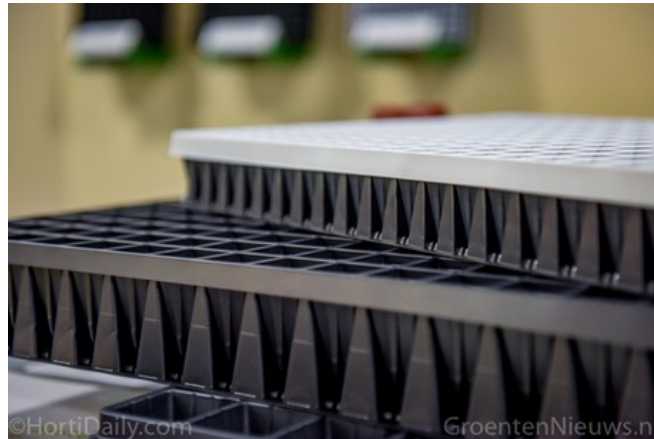
The two trays: the insert tray gives the upper cell tray a lot of strenght.
